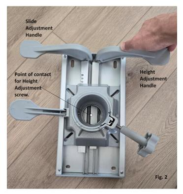
3. The pedestal sinks to the lowest point when weight is applied without the air ride handle being activated or it is stuck in the down position. The problem is the adjustment screw is too low so that it can not be activated when the adjustment handle is engaged.
